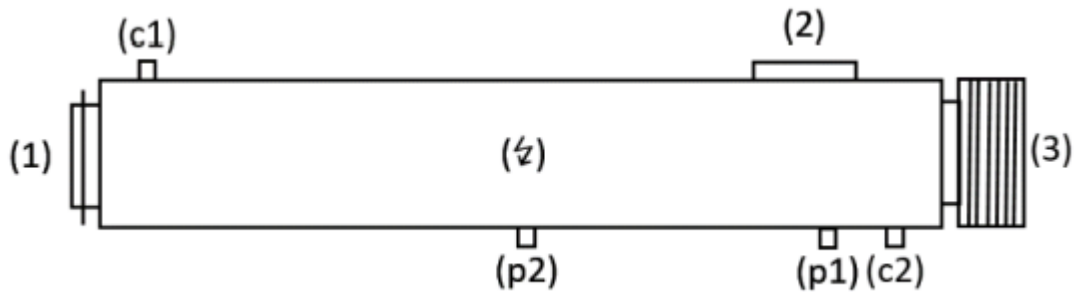
Fig. 4.3.2.3.1-2 2 Configuration with ERD (3) mounted at the front end of the test vessel
