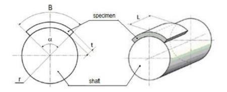
Fig. 6.13.3.3.1 Dimensions of testing specimen: r — shaft radius;  $\alpha$  — 50 °; t — specimen thickness; L — specimen length; L = 2B, mm; B — specimen width;  $B = (\pi/180) \cdot r \cdot 50$ , mm
