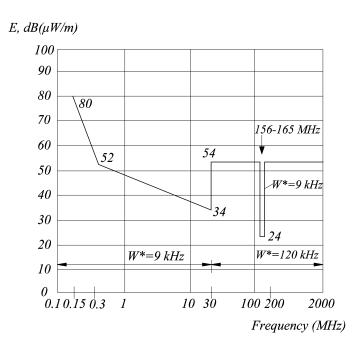
Fig. 5.1.43.2 Curve of the permissible intensity level of radiated interference field measured at a distance of 3 m from the equipment casing:  $W^*$  is the meter bandwidth
