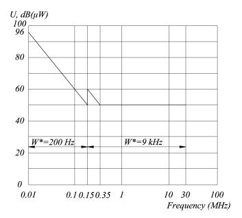
Fig. 5.1.43.1 Curve of the permissible level of conducted interference voltage U, measured at the electric power supply terminals:  $W^*$  is the meter bandwidth
