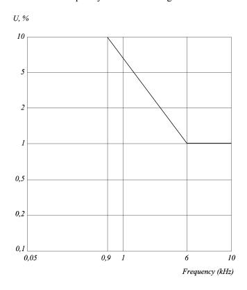
Fig. 5.1.43.3.2 Curve of the test voltage used to check the equipment for immunity to low-frequency conducted interference
