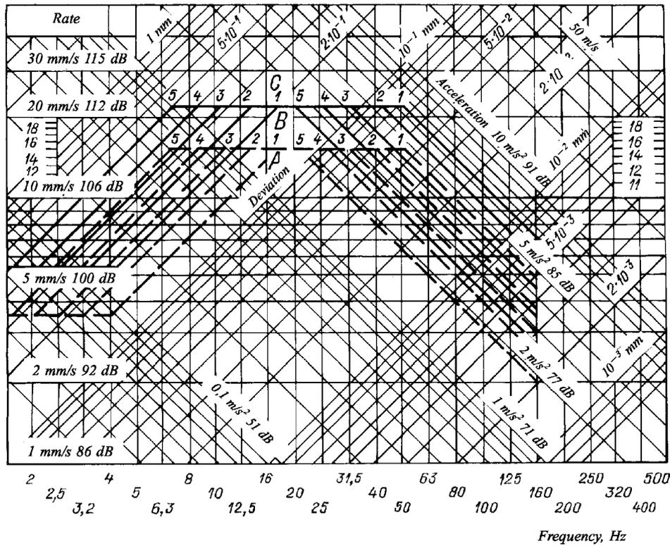
Fig. 9.3.2 Vibration standards for internal combustion engines with a piston stroke:
