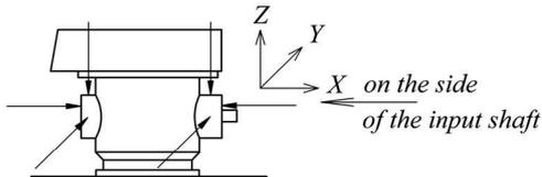
Fig. 9.9.2 Points of vibration measuring of azimuth thrusters
