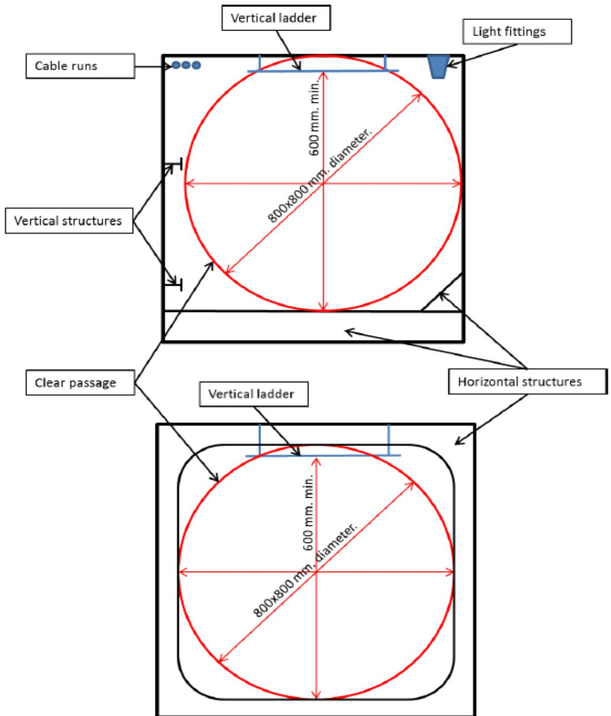
Fig. 4.5.5 Example of possible arrangements of escape fitted with a hatch taking into account minimum internal dimensions of clear width
