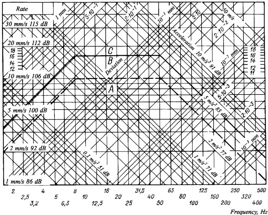
Fig. 9.6.1 Vibration standards for piston compressors:
