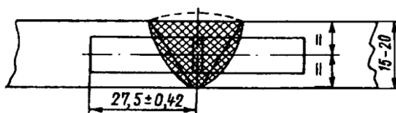
Fig. 4.8.4.1-1 Plan of V-notch specimens cutting out
