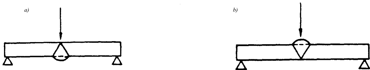
Fig. 4.4.4.4-2 Diagram of fracture testing on the root reinforcement side (a) and on the face side (b) for test specimens from the test piece P 3 , P 5 and P 6 of butt pipe joints
