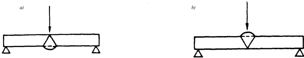
Fig. 4.4.4.4-2 Diagram of fracture testing on the root reinforcement side (a) and on the face side (b) for test specimens from the test piece P<sub>3</sub>, P<sub>5</sub> and P<sub>6</sub> of butt pipe joints
