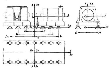
Fig. 7.1.3 Vibration isolated machine unit
