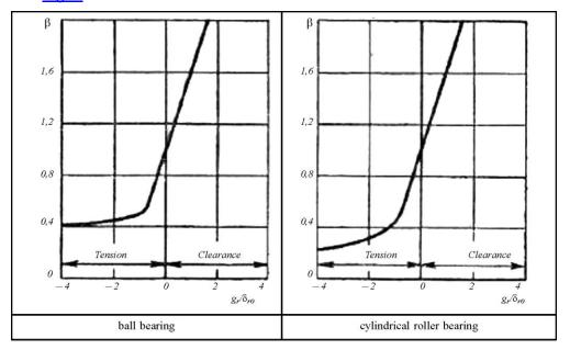
Fig. 2 Determination of factor β for
