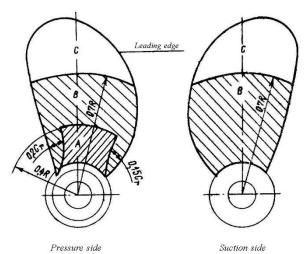
Fig. 2.1 Subdivision of the blade surface into zones: R – propeller radius;  $C_{r-}$  chord length on radius
