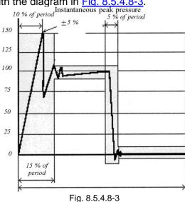
Fig. 8.5.4.8-3 Impulse pressure diagram
