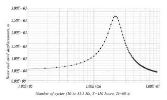
Fig. 3.3.3 Vibration amplitude variation during resonance (continuous loading)
