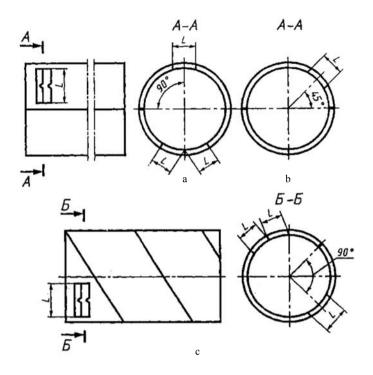
Fig. 1.1 Specimen cut out: a – longitudinal welded pipe with one longitudinal seam; b – longitudinal welded pipe with two longitudinal seams; c – spiral welded pipe; L is a specimen length
