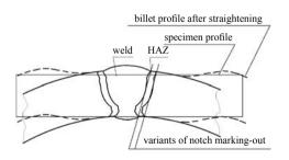
Fig. 5.4.4.3 Marking-out of pipe specimens
