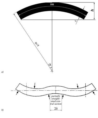
Fig. 2.1 Transverse pipe billet straightening
