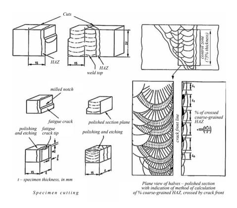
Fig. 5.4.4.8 Metallographic examination after tests
