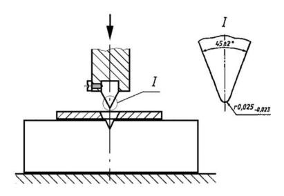
Fig. 1.3 Notch pressing-in device
