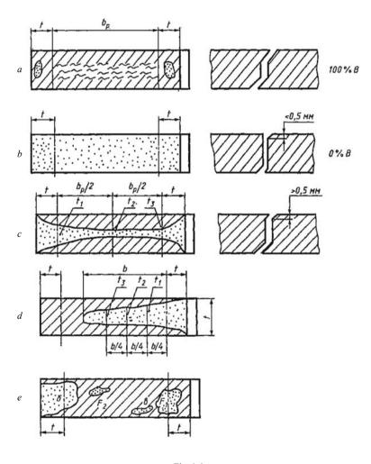
$Fig. \ 1.4$  The procedure of determining the crystalline section area and fiber percentage
