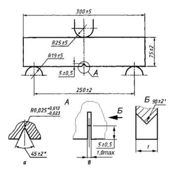
Fig. 1.2 Specimen and testing equipment (*t* – thickness)
