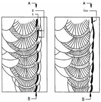
a) double heated between change points (1) and at subchange point (2) in coarse-grained  $\rm HAZ$
