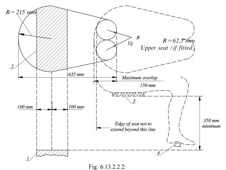
1 — lower seat; 2 — minimum seat area extends 100 mm to both sides of half-circle base line and to full width of Figure; 3 — upper seat; 4 — footrest
