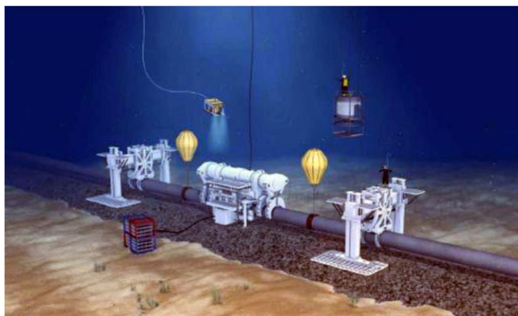
Fig. 12.2.1 Repair system of Nord Stream pipeline using Hyperbaric Welding System
