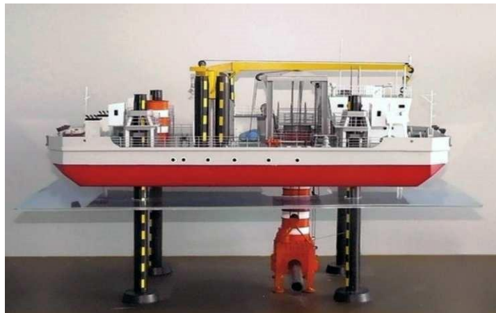
Fig. 12.3-3 Offshore Pipe Repair Platform (project 91030)
