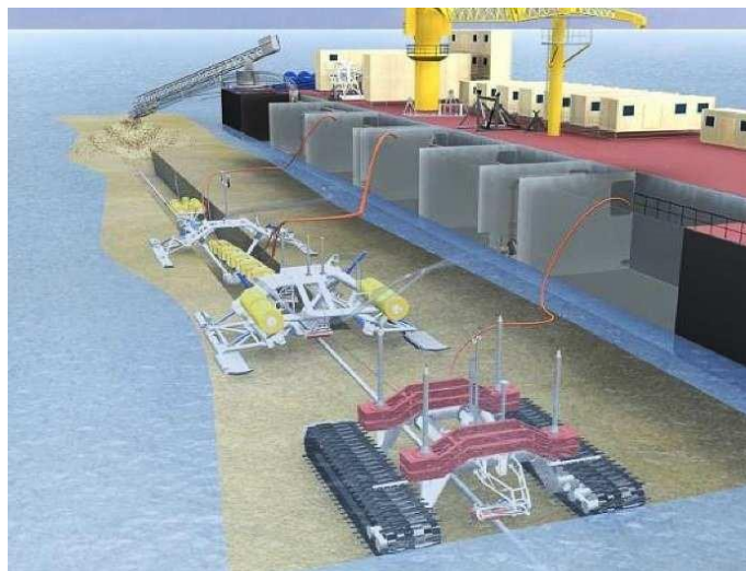
Fig. 7.6-3 Combined system for post-trenching and backfilling of a subsea pipeline developed by Saipem S.p.A.
