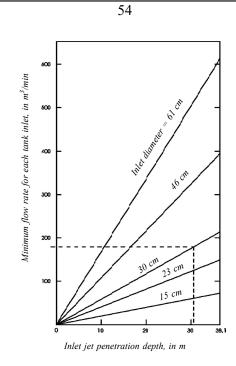
Fig. 4.3.7 Minimum flow rate as a function of jet penetration depth
