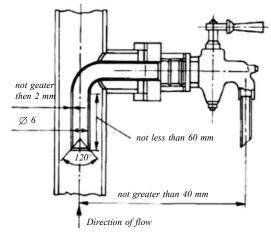
Fig. 5.2.12 Sampling arrangement for pressure piping
