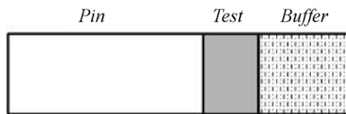
Fig. 7.2.5.4.7 Buffer and test piece location
